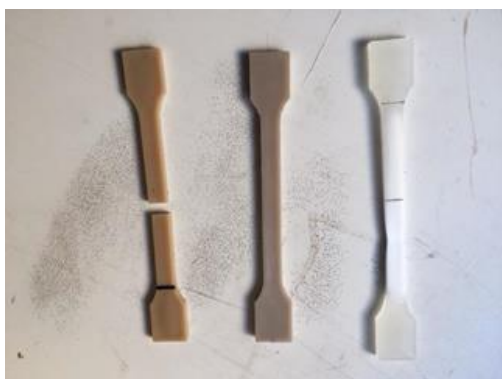
CNF mixed Plastic test pieces
